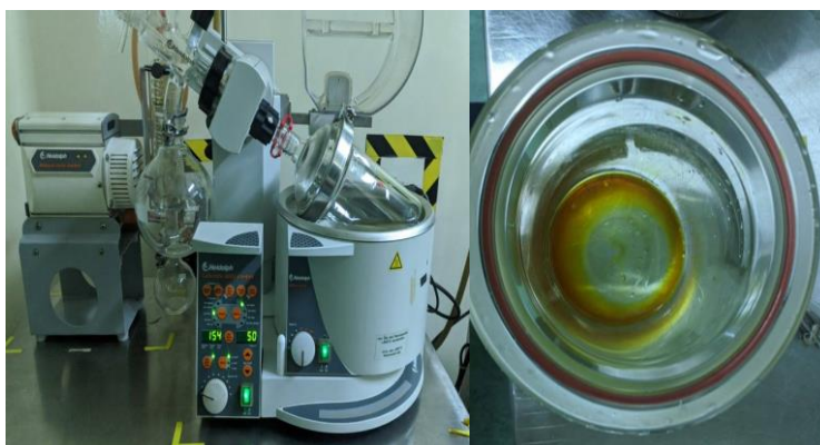
Figure 2. Gingerol separation from the solvent using Heidolph Laborota 4003
