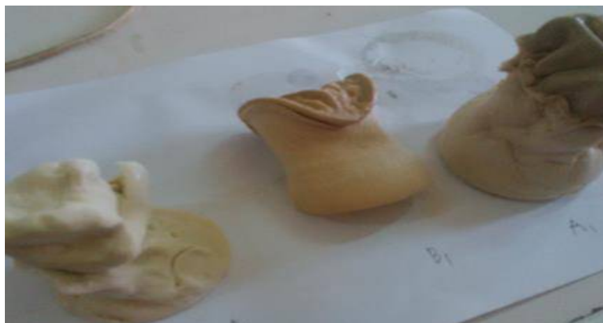
Figure 9. The Failure of Polyurethane Foam in the absence of expanding reagent
