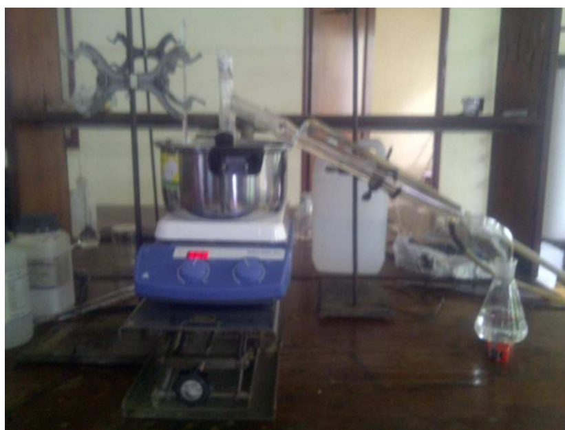
Figure 4.3: Experimental setup for hydrochlorination glycerol to 1,3-dichloropropanol
