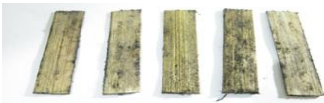
Figure 1: Bamboo fiber without Alkaly Treatment
