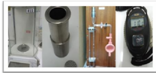
Figure 2 Blaine Testing Mechanism
