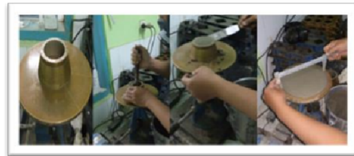
Figure 1 Mortar Workability Test
