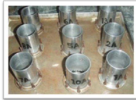
Figure 3 Cylindrical sieve with 45\mu\text{m} pore diameter
