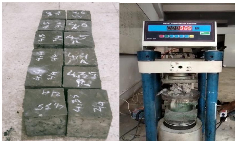
Figure 1. Test object and 4% alkaline activator geopolymer concrete.
