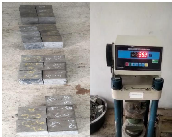
Figure 3. Compressive test of 5% alkaline activator geopolymer concrete aged 28 days.
