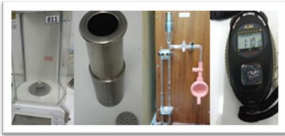
Figure 6 Blaine testing mechanism
