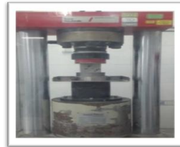
Figure 4 Compressive strength test equipment
