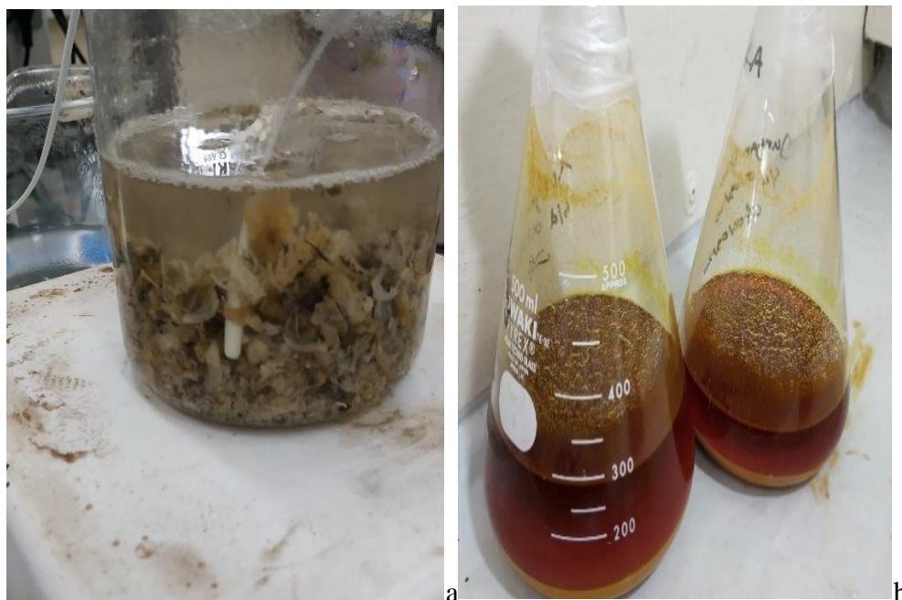
Figure 6. The extraction of catfish bone with Aquadest 70°C for 5 hours b) The maceration extraction of turmeric with methanol 96%
